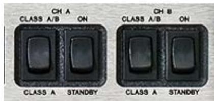
11. CLASS A/AB - Up = Class AB power tube operation (62 watts/channel). Down = Class A (Cathode Bias) power tube operation (50 watts/channel).
