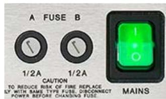
13. FUSE A - 1/2 amp fast blow fuse for Channel A
