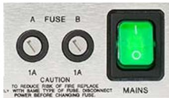
14. FUSE - 1 amp fast blow fuse for protection of individual channels.
