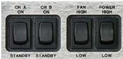
11. STANDBY - In standby, the amplifier output is disabled while power is supplied to the tube filaments only. Use STANDBY instead of the power switch during breaks to extend tube life and avoid the warm-up delay.
