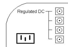
The top output delivers 12VDC @ 150mA. Outputs 2, 3 and 4 each deliver 9.5VDC @ 80mA.
